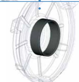
From type 90, a steel insert is provided in the bearing slot of the aluminum flanges, to resist to radial mechanical forces with a fair degree of security
