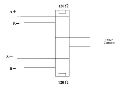
**Connecting Diagram of Terminal Resistance**
