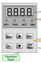
LED shows running frequency, flashing target frequency, function code, parameter value or fault code.
