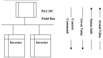
**Connecting Diagram of Field Bus**
