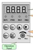
LED shows running frequency, flashing target frequency, function code, parameter value or fault code.
