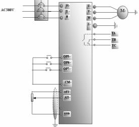
Figure 4-3 Wiring Diagram 3
