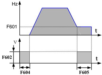
Figure 9-2 DC Braking
