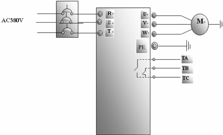
Figure 4-1 Wiring Diagram 1
